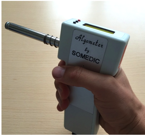
Figure 7: Handheld algometer with a 1 cm 2 probe which is placed perpendicular on the skin.
