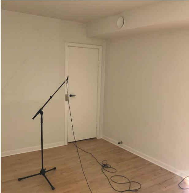
Figure 4. Photo of the living room with supply air grille and the SBi217 microphone position.
