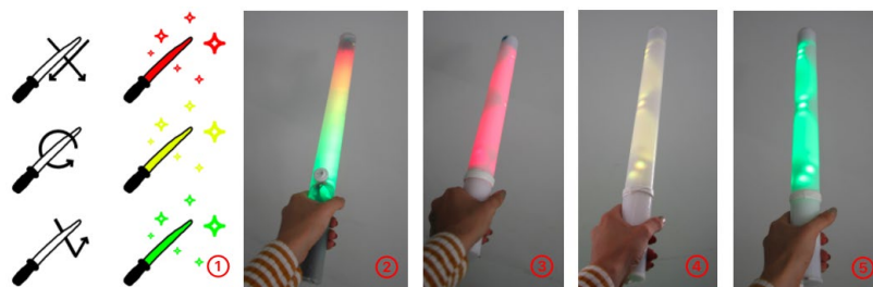
Figure 4. Glowing Wand experience prototype (1. Gesture designs; 2. Switch for a rainbow feedback; 3. Negative tick gesture to red light; 4. Circle gesture to yellow light; 5. Tick gesture to green light)
